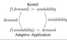
**Figure 1.** Adaptive applications create a positive-feedback loop when managed according to working set principles. Although the system may stabilize, no mechanism ensures that it converges to a configuration with maximum utility.
