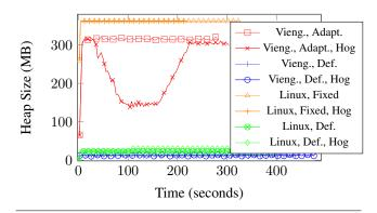
**Figure 5.** Time vs. heap size for Viengoos and GNU/Linux, using either the adaptive, fixed or default scheduler, and with or without a memory hog.
